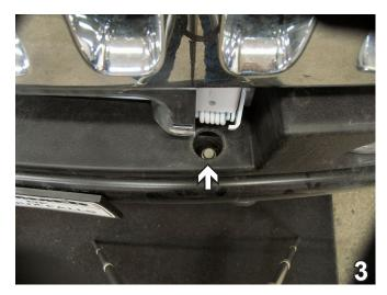
Using the 18MM socket, remove one metric bolt from the top of the bumper. Do this to both sides of the vehicle. Set bolts aside to be reinstalled later.
