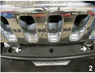
Remove the two rubber inserts from the top of the bumper. Set the rubber inserts aside to be reinstalled later.
