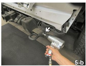
5. Using the 18MM socket, remove three metric bolts from the tow hook, two on the inside (see photo 5-a) and one on the outside (see photo 5-b). Pull tow hook forward and set aside. Do this to both sides of the vehicle. The tow hooks will not be reinstalled. Please return them to the customer.
