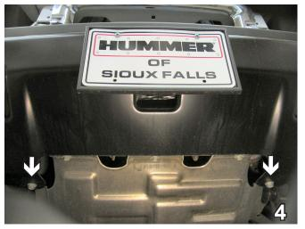
4. Just below the bumper, remove two metric bolts with the 18MM socket. Pull the metal bumper forward and disconnect the fog lights. Set bolts and metal bumper aside to be reinstalled later.
