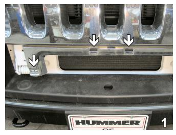
Pull the center grill insert forward to release the four clips, one on each side and two in the middle. Set insert aside to be reinstalled later. The passenger's side is shown in the photo above.
