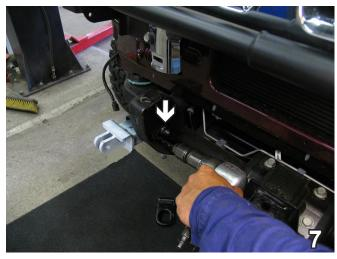
7. Using the baseplate weldment as a template, drill through the forward existing hole on the inside of the frame rail with the right angle drill and the 17/32" drill bit. Do this to both sides of the vehicle. If a right angle drill is not available, it may be necessary to remove the winch bracket to allow room for drilling.
